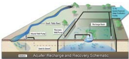
The Aquifer Recharge and Recovery System prevents the water from spilling out into the groundwater that doesn’t belong to the city of Aurora.
