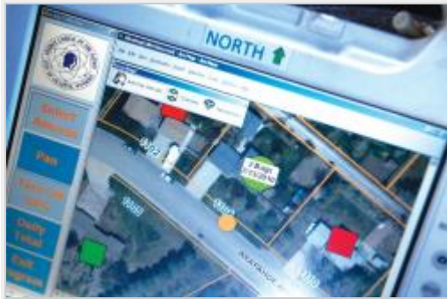
Sander Sanitation driver John Koke uses a touch book GPS to record data throughout his route. As Koke makes a stop, the touch book displays Koke's location. He will select the address and enter the amount of recyclable material collected at the home. - News-Record photo by Joy Lewis
