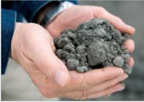
Greg Hager, vice president and general manager of the Neil Simpson complex at Wyodak, holds a pile of coal ash in his hands at Wyodak. The ash is what is left after coal is burnt and can be used as an addition to a variety of substances like concrete or asphalt. - News-Record photo by Sarah Voegele
